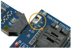
Figure 15. Switch in the OFF Position
