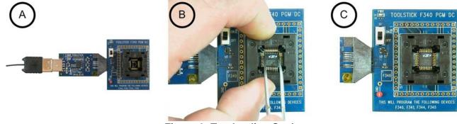
Figure 9. Top-loading Socket
