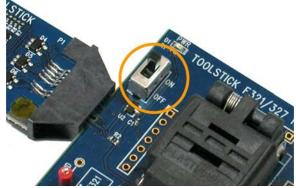
Figure 11. Switch in the ON Position
