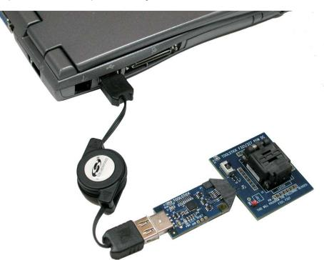
Figure 5. ToolStick Socket Platform Connected to PC Step 2. Move the switch on the daughter card to the OFF position.
