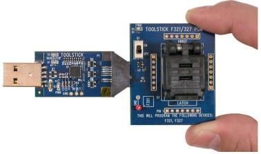
Figure 1. Proper Method of Holding the ToolStick
