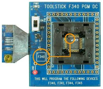
Figure 7. Socket Orientation
