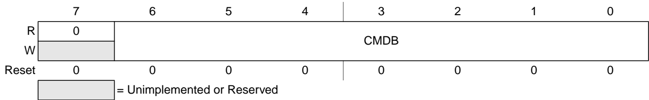
Figure 2-12. Flash Command Register (FCMD - NVM User Mode)
