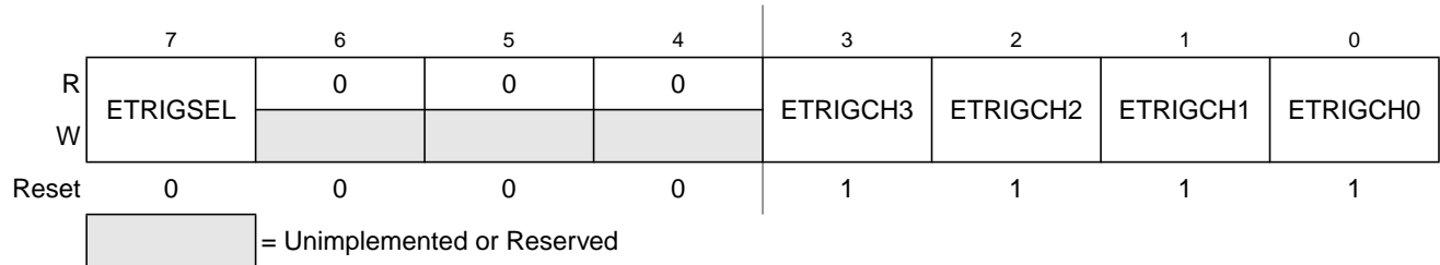
Figure 7-4. ATD Control Register 1 (ATDCTL1)
