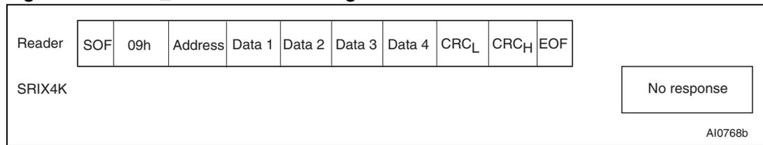
**Figure 61. Get\_UID frame exchange between reader and SRIX4K**
