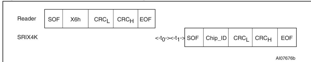
**Figure 56. Select frame exchange between reader and SRIX4K**
