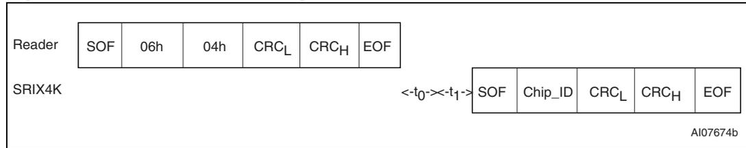
**Figure 55. Slot\_marker frame exchange between reader and SRIX4K**
