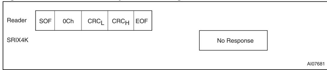
**Figure 59. Read\_block frame exchange between reader and SRIX4K**
