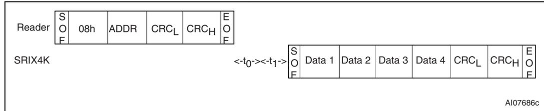
**Figure 60. Write\_block frame exchange between reader and SRIX4K**
