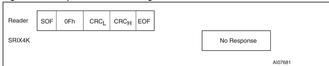
**Figure 58. Reset\_to\_inventory frame exchange between reader and SRIX4K**
