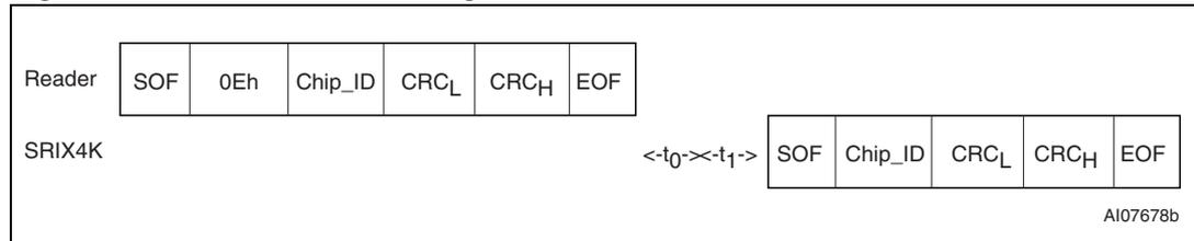
**Figure 57. Completion frame exchange between reader and SRIX4K**
