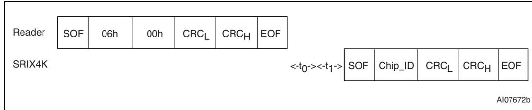
**Figure 54. Pcall16 frame exchange between reader and SRIX4K**
