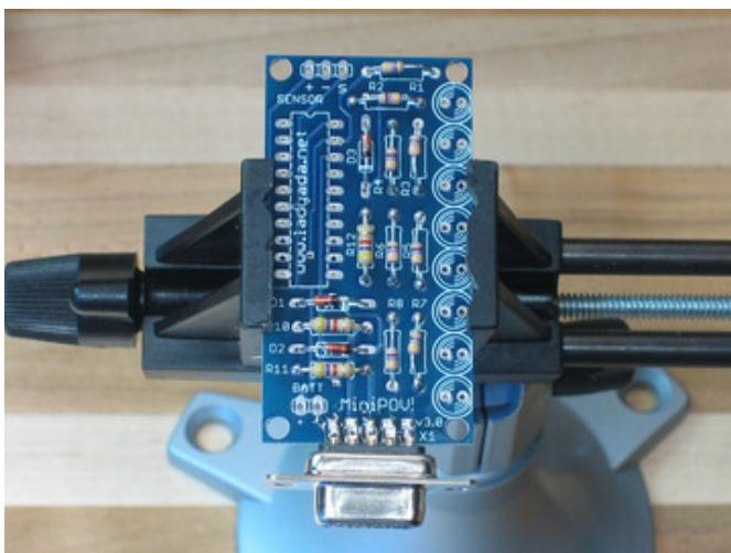
On the other side, solder and clip the diodes and solder the other 4 pins of the serial port connector.
