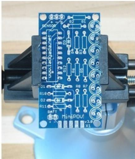
Put the circuit board in the vice, ready for soldering!
