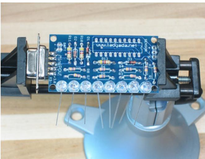
For the next step, you will place the 8 LEDs. LEDs have a 'direction' so if they're backwards they don't work. There are three ways to tell the direction.
