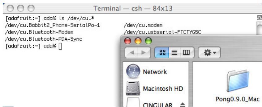
If you're using an FTDI-chip based adapter, it will show up as `/dev/cu.usbserial-FTCxxxx`. If you're using a PL2303 chipset adapter, it'll show up as `/dev/cu.PL2303-1B1`
