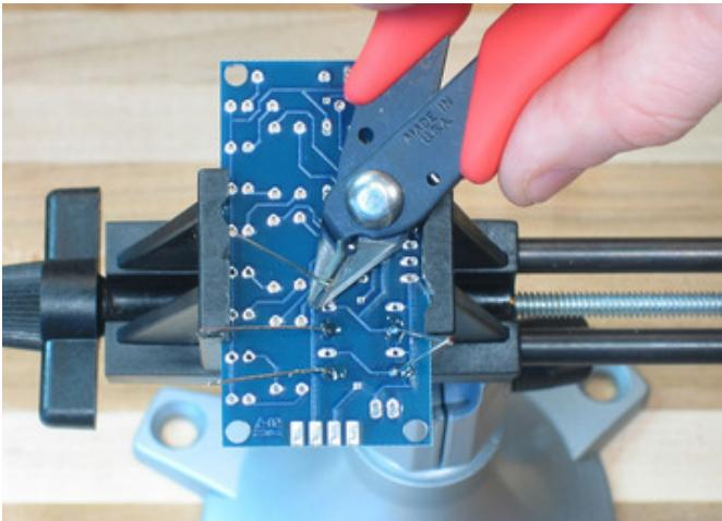
Cut the leads off so that only the blob remains. Be careful, the wires can fly out at you!
