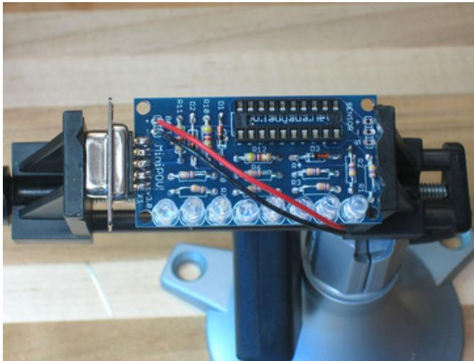
Solder in the two battery holder wires, red is + and black is -
