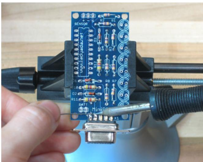
Start by soldering on the serial port connector. Make sure that you're actually soldering the pins to the circuit board (solder underneath) rather than just filling the pins with solder.
