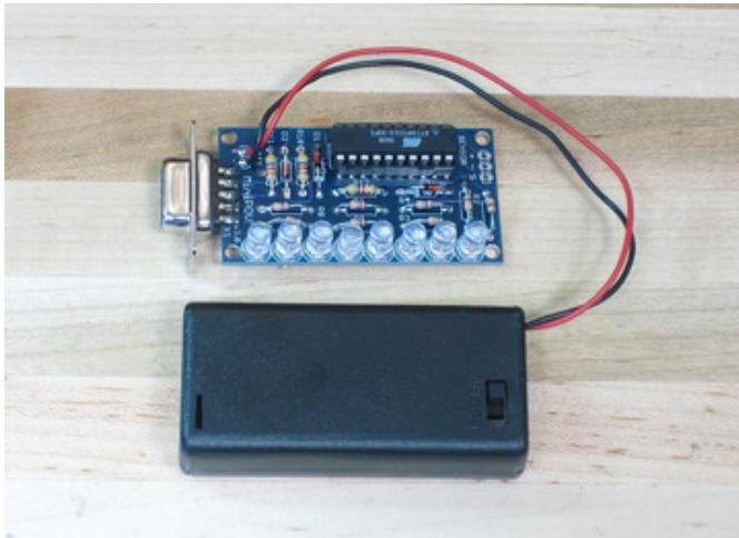
Place the microcontroller in as shown and put in 2 AA batteries, be sure to turn it on with the switch!
