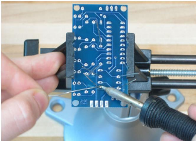
Make sure your solder iron is hot, hold it with your dominant hand. Use the other hand for guiding the solder in. Now steady your hands so that you can touch the very hot tip of the iron to the lead (resistor wire) and pad (circuit board hole) at the same time. Heat the two for 2 counts then dip the solder in, you should get a nice shiny blob as shown.
