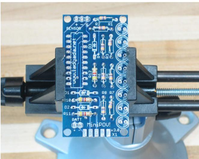
Place the 8 47 ohm resistors, just like the last time.
