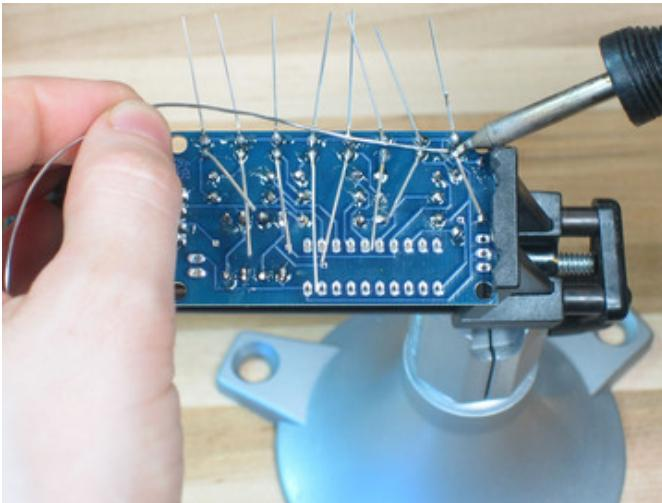
Turn the board over and solder in the LEDs, then clip the leads.
