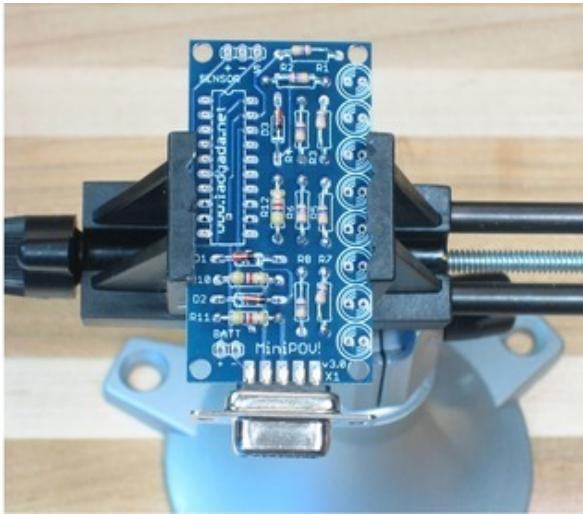
Place the three zener diodes and the serial port connector. The diodes are directional so don't put them in backwards. Note that there is a black stripe on the red glass, this stripe matches the white stripe on the silkscreen picture of the diode.
