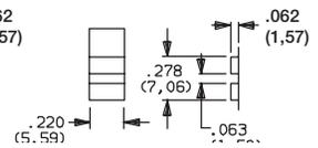
**NOTE:** Standard actuator color is black, other colors available, consult Customer Service Center. Alternate heights are available with '03, 04 and 09' actuators, consult Customer Service Center. Models with S2 mounting style, subtract .090 (2,29). Actuators '12' and '13' are available with DPST and DPDT models only.
