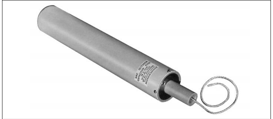
Figure 1. NXC outdoor capacitor fuse, available in voltage ratings of 8.3, 15.5 and 23 kV, offers positive leader wire ejection for reliable interruption and elimination of electrical stress to circuit apparatus. Top end cap has provision for convenient bus bar mounting.
