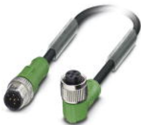
Sensor/actuator cable, 5-position, PUR halogen-free, black-gray RAL 7021, Plug straight M12, A-coded, on Socket angled M12, A-coded, cable length: 1.5 m
