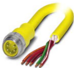
Sensor/actuator cable, 5-position, PVC, yellow, Plug straight 7/8"-16UNF, A-coded, on free cable end, cable length: 6 m
