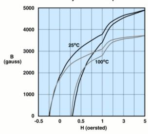
Measured on an 18/10/6mm toroid at 10kHz.
