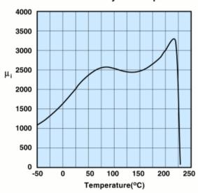
Measured on an 18/10/6mm toroid at 100kHz.
