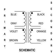
$<sup>^{1}\,</sup>$  Primary and secondary windings are designed to be connected in series or parallel. Windings are not intended to be used independently.
