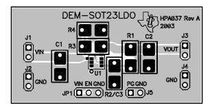
Figure 1. Assembly Layer
