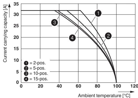
The figure shows the derating curve of the UT 4/1P... terminal block in connection with the UPBV 4 plug
