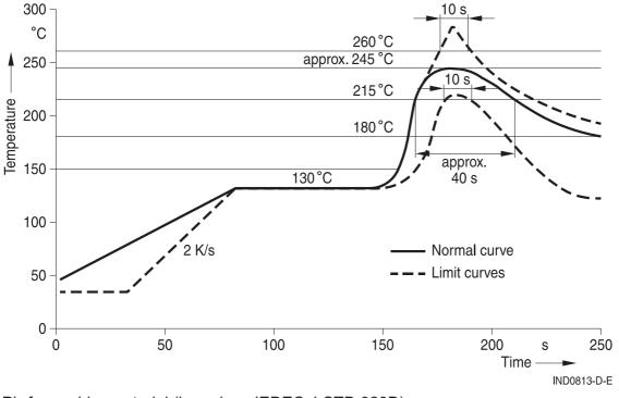
Pb-free solder material (based on JEDEC J-STD 020D)
