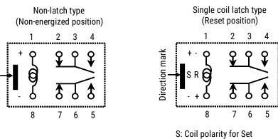
R: Coil polarity for Reset
