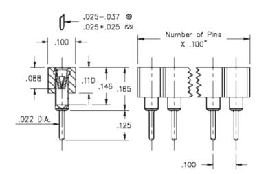
Interconnect Socket Standard Solder Tail Socket Accepts .025"- .037" (0,635 - 0,94 mm)dia leads Single Row Through Hole Plating Code: 43 Shell Plating: 200 µ" Tin (matte finish) over 100 µ" Nickel Inner Contact Plating:
