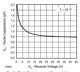
Fig. 2 - Diode Capacitance vs. Reverse Voltage
