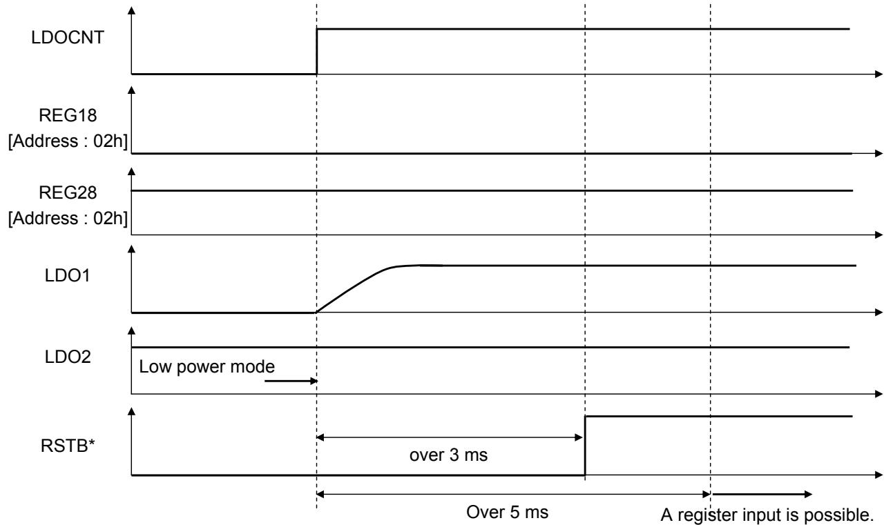
\* It is a waveform in the case of applying reset to register setup at Standby mode.
