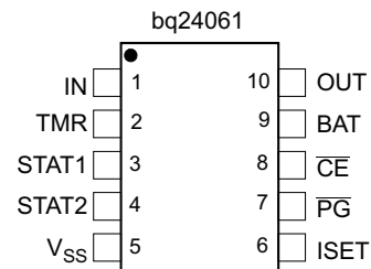
Pin Out (Top View)
