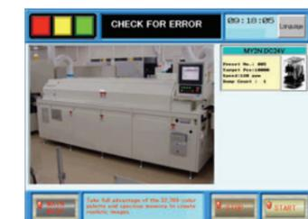
When an error occurs, the location of the error can be shown realistically in a picture.
