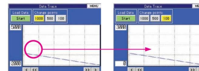
Any position from the host (PLC) can be plotted as a graph.
