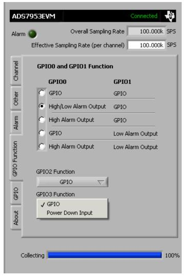
Figure 23. GPIO and System Monitor Control options
