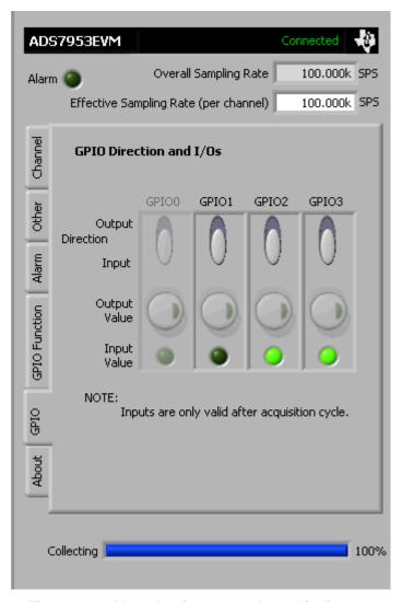
Figure 24. GPIO selection, controls and indicators
