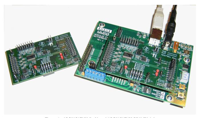
Figure 1. ADS7953EVM (Left) and ADS7953EVM-PDK (Right)
