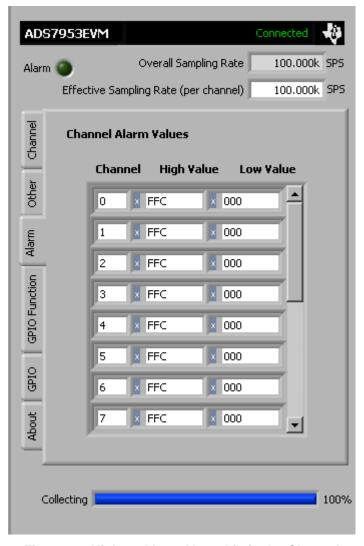
Figure 22. High and Low Alarm Limits by Channel
