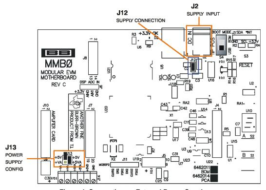
Figure 4. Connecting an External Power Supply
