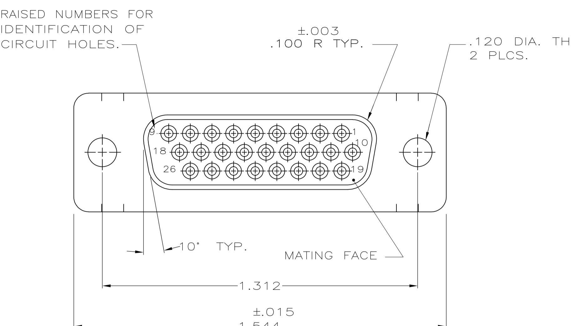
1. THIS RECEPTACLE WILL MATE WITH ANY SIZE 2,26 POSN. PLUG IN AMPLIMITE SERIES.
