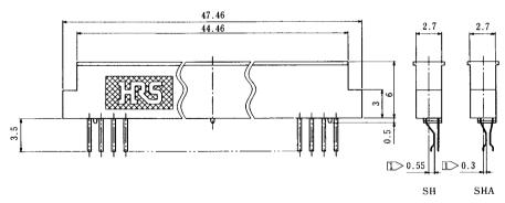
• Recommended board thickness: 0.4 to 0.5mm
