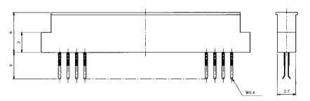
• Recommended board thickness: 0.4 to 0.5mm
