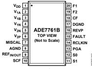
Figure 3. Pin Configuration (SSOP)
