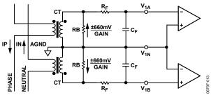
Figure 15. Typical Connection for Channel V1
