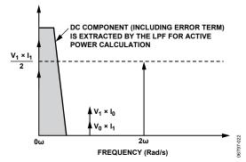
Figure 24. Effect of Channel Offsets on the Active Power Calculation
