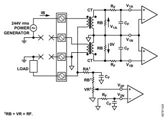
Figure 31. Missing Neutral System Diagram
