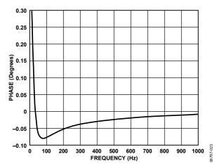
Figure 25. Phase Error Between Channels (0 Hz to 1 kHz)
