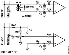
Figure 16. Typical Connections for Channel V2
