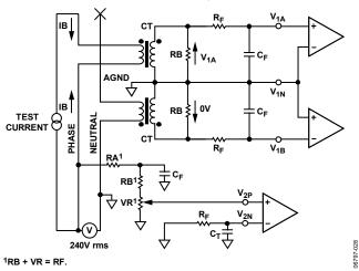
Figure 30. Conditions for Calibration of Channel B
