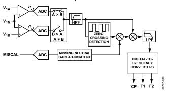
Figure 32. Energy Calculation in Missing Neutral Mode
