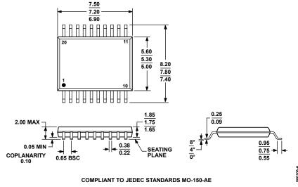
Figure 36. 20-Lead Shrink Small Outline Package [SSOP] (RS-20) Dimensions shown in millimeters
