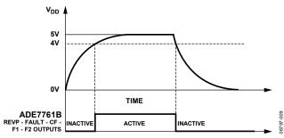
Figure 11. On-Chip, Power Supply Monitoring
