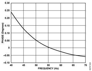
Figure 26. Phase Error Between Channels (40 Hz to 70 Hz)
