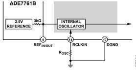
Figure 18. Internal Oscillator Connection
