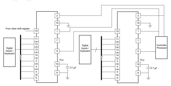
Figure 5. Typical Application Diagram for SN74HC165
