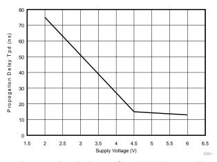
Figure 6. Propagation Delay vs Supply Voltage at T<sub>A</sub> = 25°C
