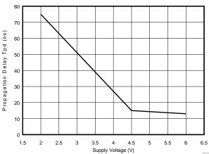
Figure 1. Propagation Delay vs Supply Voltage at  $T_A = 25$ °C
