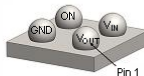
Figure 4. WLCSP Bumps Facing Up (Bottom View)
