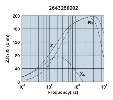
Impedance, reactance, and resistance vs. frequency.
