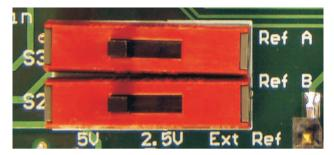
Figure 4. Default Settings for Switch S2 and S3
