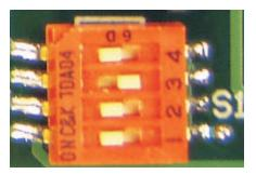
Figure 3. Default Settings for Switch S1 (LDAC Low)
