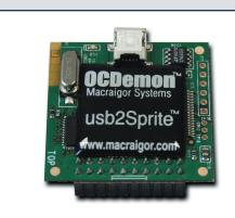
The usb<sup>2</sup>Sprite is a self-powered, cable-less, miniaturized (2.25 in<sup>2</sup>) version of our usb<sup>2</sup>Demon that plugs directly into a board's JTAG/BDM header providing "built-in" debug connectivity. To the user the usb<sup>2</sup>Sprite looks like a USB mini connector sitting on top of the board's JTAG/BDM header. Problems caused by customer installation errors, JTAG cable noise, parallel port incompatibility, and the need for an external power supply are eliminated.
