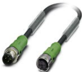
Sensor/actuator cable, 4-position, PUR, black-gray RAL 7021, Plug angled M12 SPEEDCON, A-coded, on Socket straight M12 SPEEDCON, A-coded, cable length: 2.5 m
