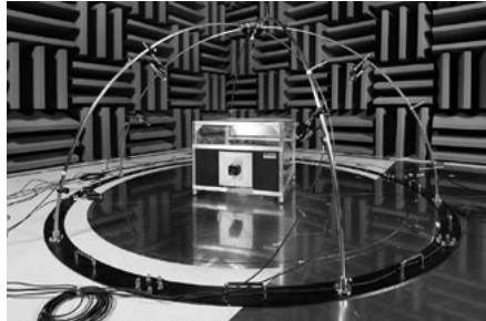
Noise characteristic measurement equipment
