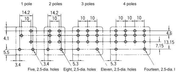
**Note:** The figures and dimensions depicted here are for the LY2-0. The dimension with an asterisk (\*) is 6.4 for the LY1-0.
