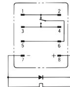
(Check the coil polarity when wiring and wire all connections correctly.)
