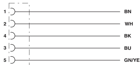
Contact assignment of the M12 sockets
