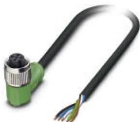
Sensor/actuator cable, 5-position, PVC, black RAL 9005, free cable end, on Socket angled M12, A - standard, cable length: 2 m
