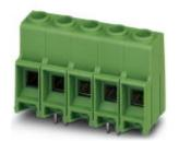
PCB terminal block, nominal current: 76 A, nom. voltage: 1000 V, pitch: 10.16 mm, number of positions: 3, connection method: Screw connection with tension sleeve, mounting: Wave soldering, conductor/PCB connection direction: 0 °, color: green
