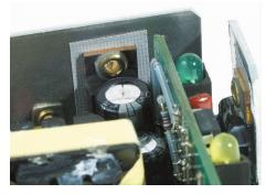
Sil-Pad<sup>®</sup> 400 is a composite of silicone rubber and fiberglass. The material is flame retardant and is specially formulated for use as a thermally conductive insulator. The primary use for Sil-Pad<sup>®</sup> 400 is to electrically isolate power sources from heat sinks.
