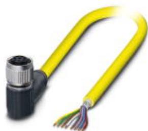
Sensor/actuator cable, 8-position, PVC, yellow, shielded, free cable end, on Socket angled M12 SPEEDCON, coding: A, cable length: 5 m
