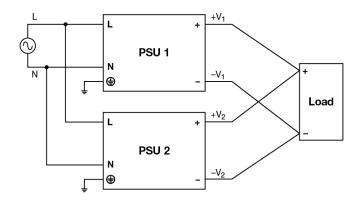
Fig. 6 Parallel Operation Connection Diagram
