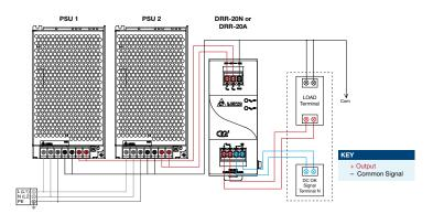
Fig. 5 Redundancy Operation Connection Diagram
