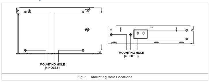
With reference to Fig. 3, the device should be mounted on a sturdy heat conducting surface with minimum of 4 mounting holes for base mounting or 3 mounting holes for side mounting. Use M3 screws only.
