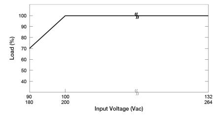
No output power de-rating for the input voltage from 100Vac to 132Vac & 200Vac to 264Vac
