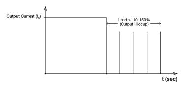
It is not recommended to prolong the duration of I<sub>O</sub> when it is <110-150% but >100%, since it may cause damage to the PSU.
