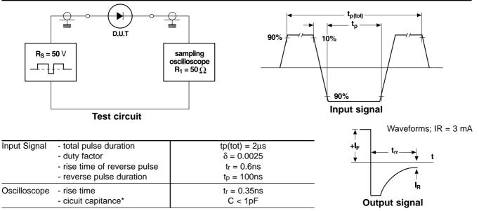
\*C = oscilloscope input capactitance + parasitic capacitance
