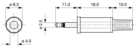
Cable diameter max. 4.0 mm
