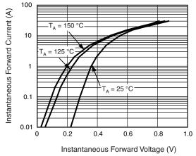
Fig. 3 - Typical Instantaneous Forward Characteristics
