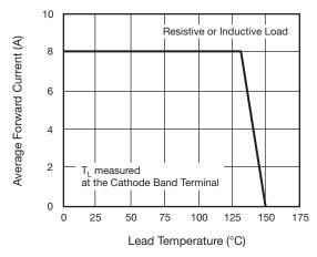
Fig. 1 - Maximum Forward Current Derating Curve
