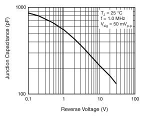
Fig. 5 - Typical Junction Capacitance
