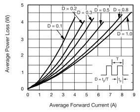
Fig. 2 - Forward Power Loss Characteristics
