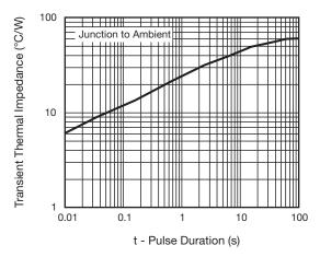
Fig. 6 - Typical Transient Thermal Impedance
