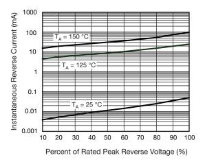
Fig. 4 - Typical Reverse Leakage Characteristics
