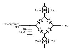
Figure 2. Timing Test Circuit
