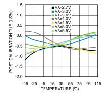
Figure 21. Max TUE vs Temperature
