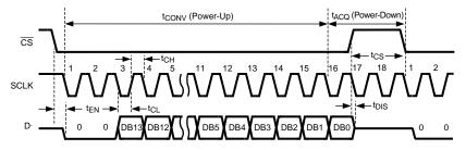
Figure 33. ADC141S628Q Single Conversion Timing Diagram
