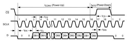
Figure 1. ADC141S628Q Single Conversion Timing Diagram
