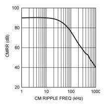
Figure 31. Analog Input CMRR vs Frequency
