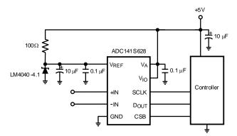
Figure 35. Low-Cost, Low-Power Data Acquisition System
