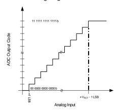
Figure 34. ADC Output vs Input
