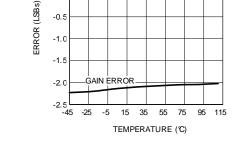
Figure 19. Gain and Offset Error vs Temperature
