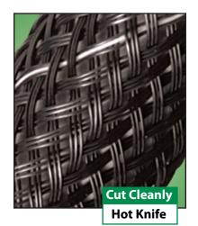
HALAR® (HT) self-extinguishing sleeving is used where flammability, high temperature endurance and low outgassing are primary concerns. HT is braided from 11 mil ethylene chlorotriflouroethylene (ECTFE) copolymer monofilament.
