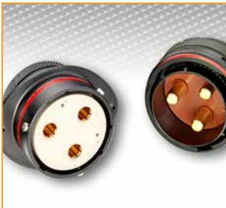
Expanding our range of ASHD power connectors, the new 3-way version is designed for 3-phase electric motors or generators to meet the growing need of hybrid racecars. The connectors use three 4 AWG contacts for power and two 20 AWG signal contacts for a safety loop.
