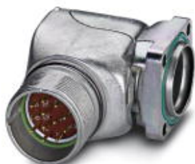
Device connector, front mounting, angled fixed, Screw locking, M23, number of positions: 16, type of contact: Pin, Crimp connection, Axial O-ring, 4x Ø 3.2, shielded: yes, flange dimensions: 28 mm x 28 mm
