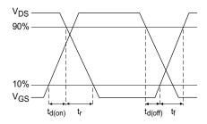
Fig. 11 - Switching Time Waveforms
