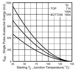
Fig. 15 - Maximum Avalanche Energy vs. Drain Current
