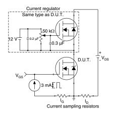
Fig. 17 - Gate Charge Test Circuit
