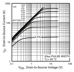
Fig. 1 - Typical Output Characteristics
