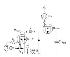
Fig. 13 - Unclamped Inductive Test Circuit
