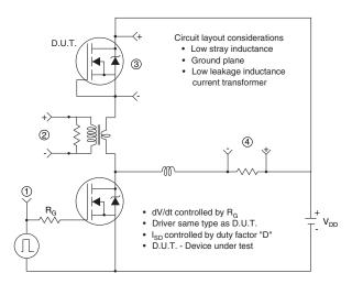
Fig. 18 - Peak Diode Recovery dV/dt Test Circuit
