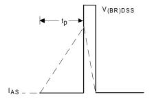
Fig. 14 - Unclamped Inductive Waveforms
