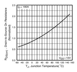
Fig. 4 - Normalized On-Resistance vs. Temperature
