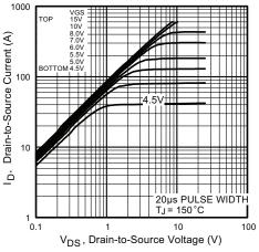
Fig. 2 - Typical Output Characteristics
