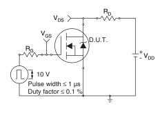
Fig. 10 - Switching Time Test Circuit
