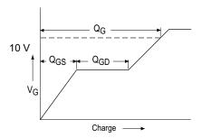
Fig. 16 - Basic Gate Charge Waveform
