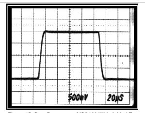
Figure 15. Step Response of ISO122 With Added Twopole Output Filter
