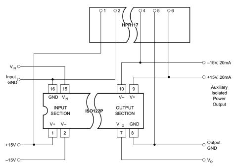
Figure 22. Input-Side Powered ISO Amp
