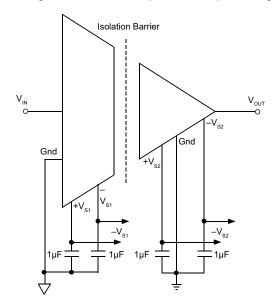
Figure 24. Basic Signal and Power Connections
