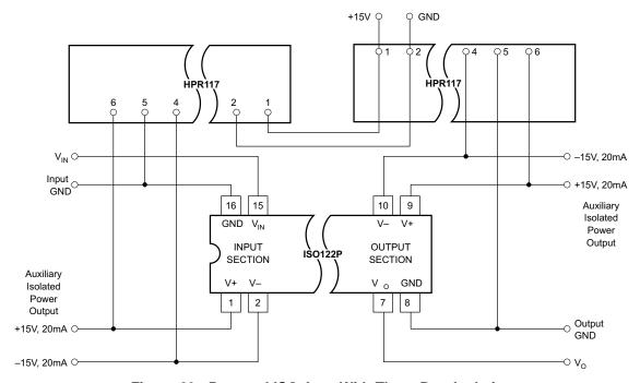
Figure 23. Powered ISO Amp With Three-Port Isolation
