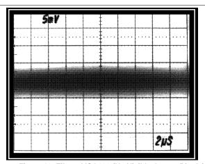
Figure 13. Filtered ISO122 (No Visible Output Ripple)
