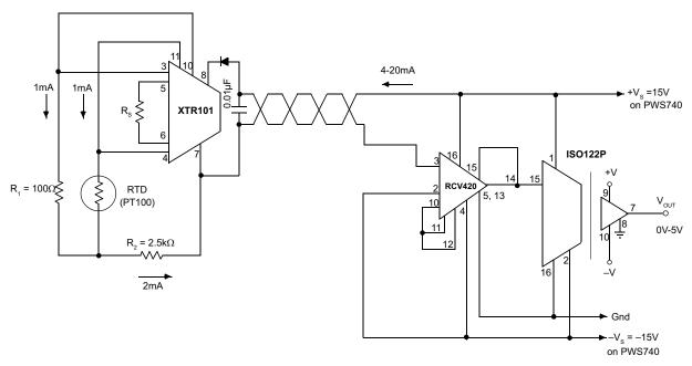
Figure 20. Isolated 4- to 200-mA Instrument Loop. (RTD shown.)
