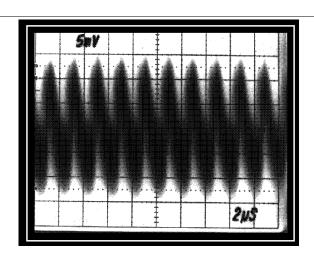
Figure 12. Standard ISO122 (Approximately 20-mVp-p Output Ripple)
