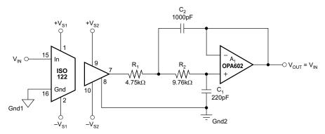
Figure 10. ISO122 With Output Filter for Improved Ripple
