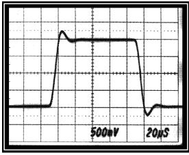
Figure 14. Step Response of Standard ISO122
