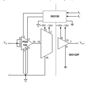
Figure 18. Programmable-Gain Isolation Channel With Gains of 1, 10, and 100
