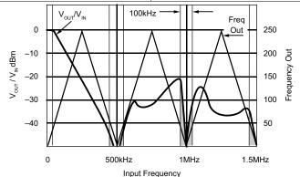
NOTE: Shaded area shows aliasing frequencies that cannot be removed by a low-pass filter at the output.
