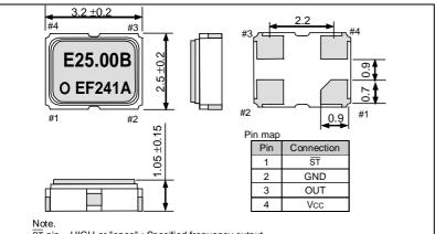
ST pin = HIGH or "open" : Specified frequency output.
