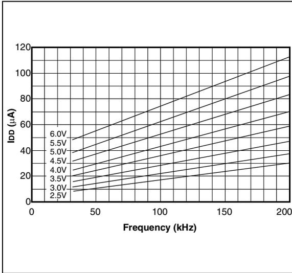
**FIGURE 14-27: TYPICAL  $I_{DD}$  vs. FREQUENCY (XT MODE, 25°C)**
