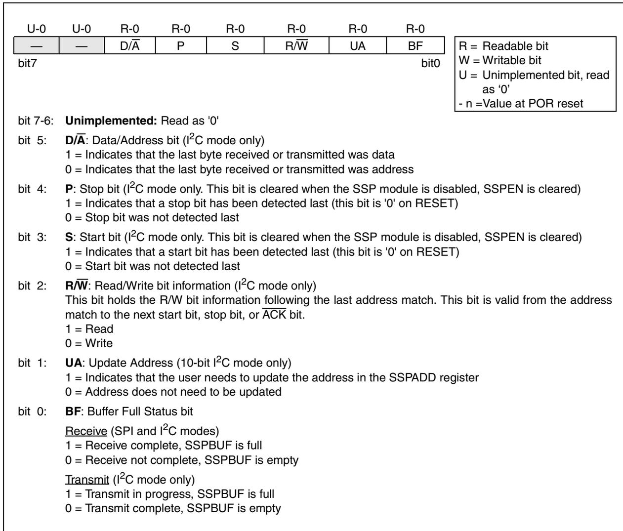
**FIGURE 8-2: SSPCON: SYNC SERIAL PORT CONTROL REGISTER (ADDRESS 14h) (PIC16C72)**
