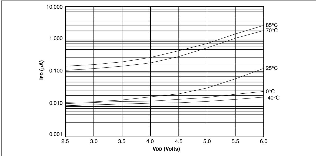
**FIGURE 14-3: TYPICAL IPD vs. VDD @ 25°C (WDT ENABLED, RC MODE)**
