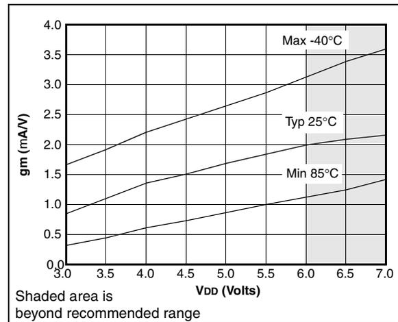
**FIGURE 14-20: TRANSCONDUCTANCE(g<sub>m</sub>) OF LP OSCILLATOR vs. V<sub>DD</sub>**
