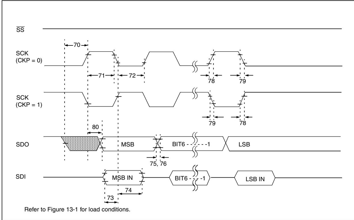
**FIGURE 13-9: SPI MASTER OPERATION TIMING (CKE = 1)**
