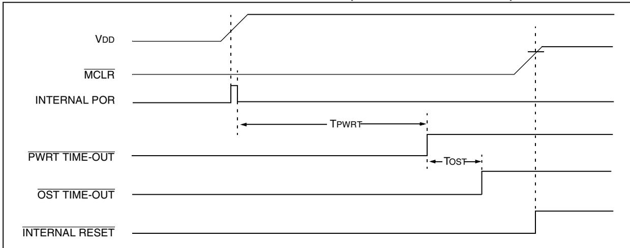
**FIGURE 10-10: SLOW RISE TIME ( $\overline{\text{MCLR}}$  TIED TO  $V_{\text{DD}}$ )**
