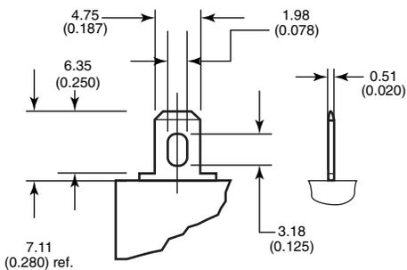
**Note:** Mates with .187" UL standard quick-connect terminals; also suitable for solder connection.
