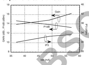
LNA - Gain, P1dB, Output IP3 vs. Current [2] @ 900 MHz
