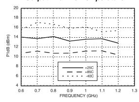
LNA - Output P1dB vs. Temperature [2]
