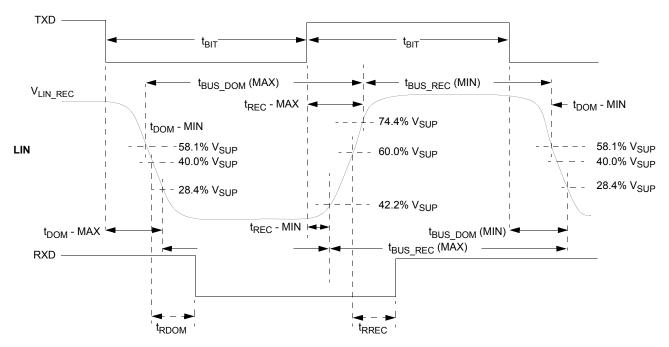
Figure 30. LIN timing measurements for normal slew rate
