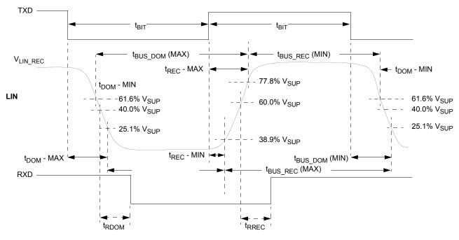
Figure 31. LIN timing measurements for slow slew rate
