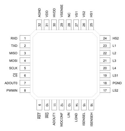
Figure 3. 33912 pin connections
