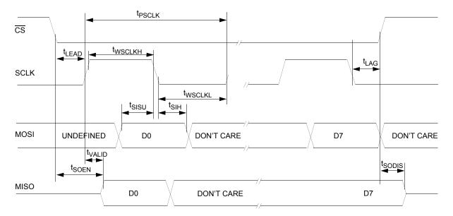
Figure 36. SPI timing characteristics
