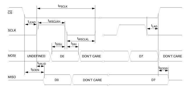
Figure 13. SPI timing characteristics
