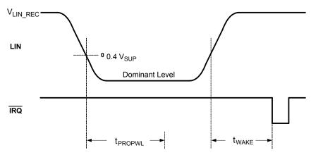
Figure 34. LIN wake-up stop mode timing
