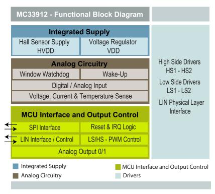
Figure 37. Functional internal block diagram
