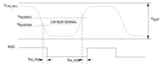
Figure 32. LIN receiver timing
