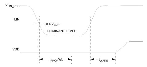
Figure 33. LIN wake-up sleep mode timing
