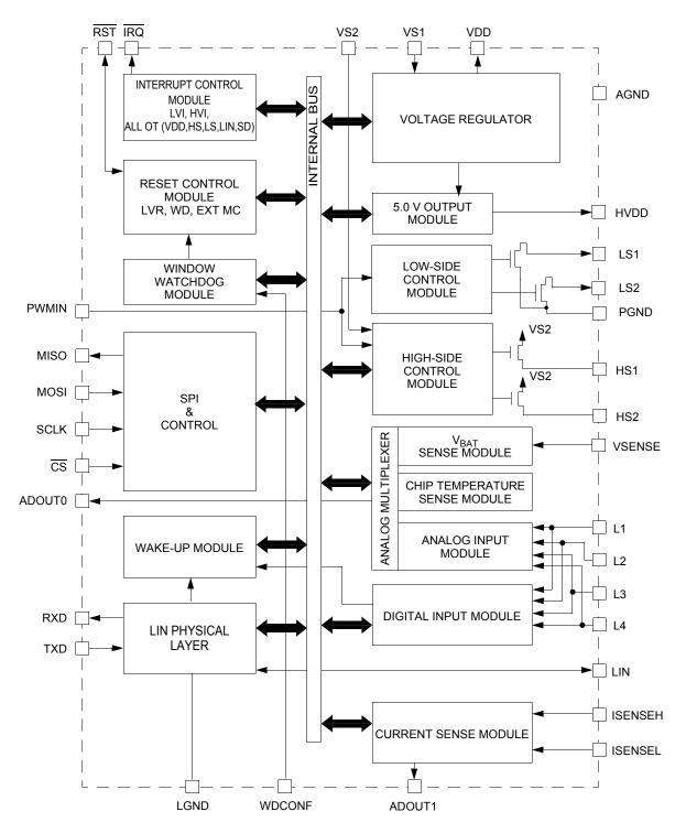
Figure 2. 33912 simplified internal block diagram
