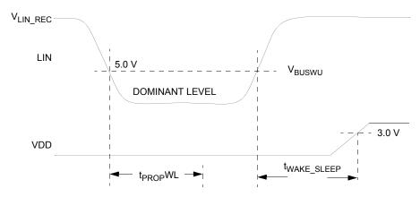
Figure 10. LIN wake-up sleep mode timing
