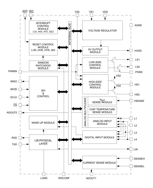
Figure 25. 33912 simplified internal block diagram
