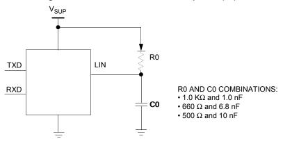
Figure 6. Test circuit for LIN timing measurements
