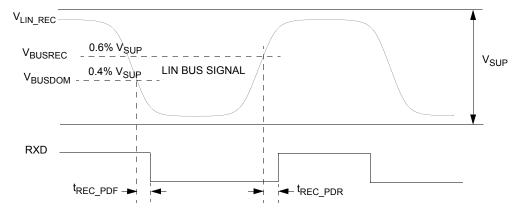
Figure 9. LIN receiver timing
