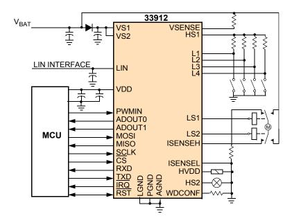
Figure 1. 33912 simplified application diagram
