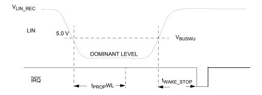
Figure 11. LIN wake-up stop mode timing
