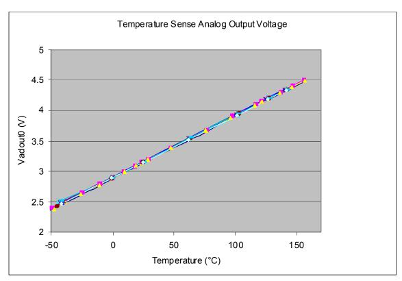
Figure 16. Temperature sense gain
